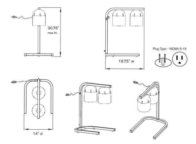
Electric: Attached 6-foot flexible, three-wire cord with ground plug (NEMA 5-15).
